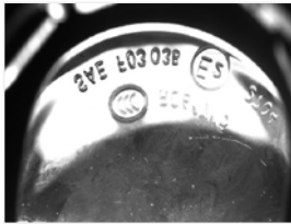
6. Inspection of letters in lampshade
