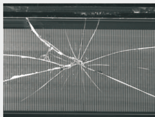
Lens surface crack detection
