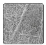
Pre filter media viewed with an electron microscope at 500 times magnification
