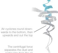
The centrifugal force separates the dust and particulate from the air
