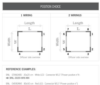
BNL OVERDRIVE 80x50 cm Red LED Connector M12 I-Power position n° Cable 2.50 meters position n°5: → BNL-0-8050-630-M1A5
