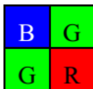
Figure 3-5 Bayer BG Pixel Pattern
