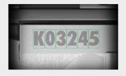
The outstanding Advanced OCR software algorithm ensures the highest reading reliability of ink-jet dot matrix characters on challenging surfaces (i.e. cans, bottles,..)
